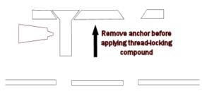
bolts. Then refit the anchor by guiding the bolts through their holes.
